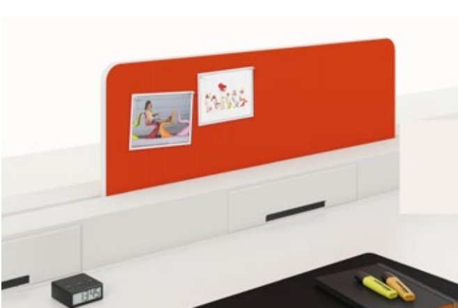
Screen with pin board: Screen with pin board for lateral separation of individual workstations. Core material made of high-density tri-ply high-grade fibreboard (conforms to EN 312) in the thickness FPY24. Both sides fabric-covered and fixed. Circumferential platform edge made of plastic.
